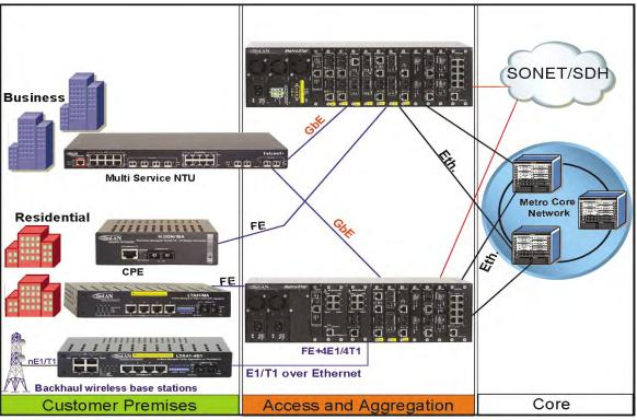
**MetroStar™** equipped with a management module can be monitored and managed from any SNMP management station running popular management platforms (e.g. FibroLAN's *MetroView*, HP OpenView. SNMPc. etc)
