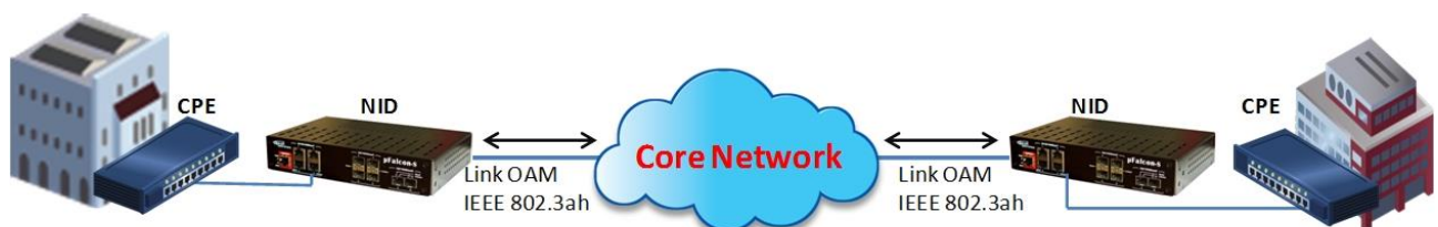
Figure 4-162: Sample Network with OAM functionality
