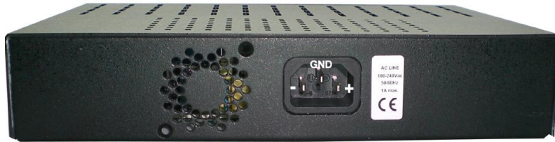
Figure 6-19: \mu Falcon-MX rear panel 125VDC connector
