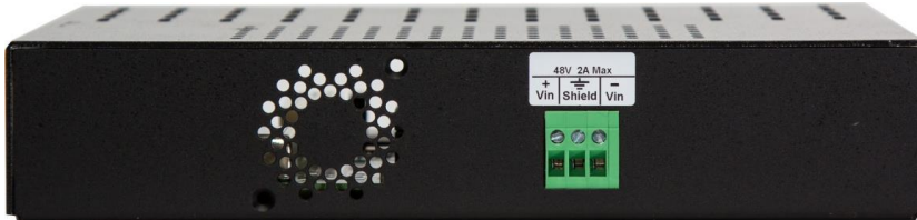
Figure 6-20: \mu Falcon-MX series DC PS rear panel ST connector
