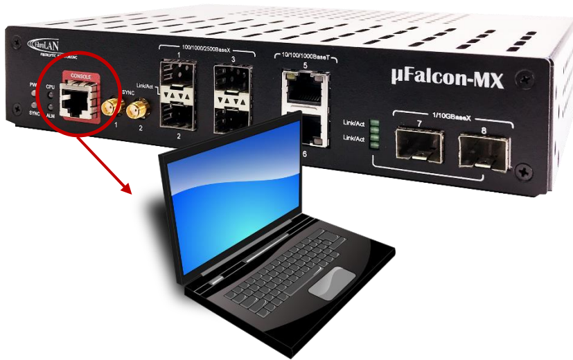
Figure 1-8: \mu Falcon-MX console connection
