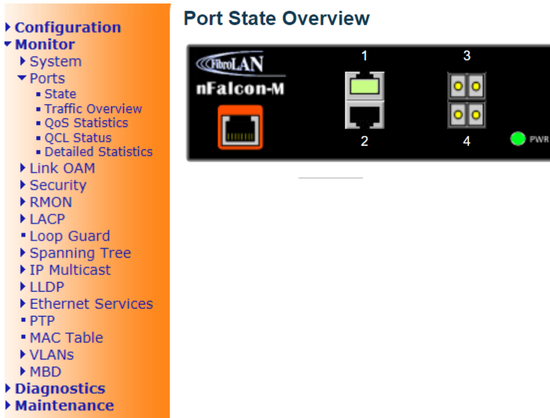
Figure 5-32: M-Class series Web management front panel overview
