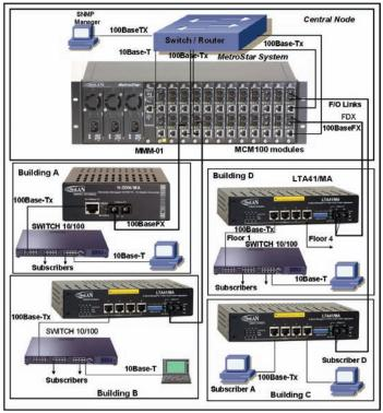
MetroStar™ equipped with a management module can be monitored and managed from any SNMP management station running popular management platforms (e.g. FibroLAN's MetroView, HP OpenView, SNMPc, etc)
